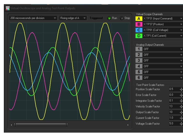
We can see approximately 20 volts peak to peak and 5 amps peak to peak flowing through the scanner coil. RMS Coil current is thus 1.77 amps.
