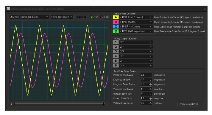
In this case we see that the RMS current being driven into the scanner is around 4.1 amps, and coil temperature is around 55C (assuming the scanner body is 30C). The scanner will be dissipating 30 watts, and power required from the power supply is around 2.25 amps per rail.
