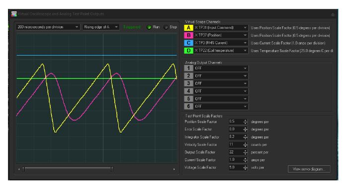
The oscilloscope shows that the RMS current being driven into the scanner is roughly 3.3 amps and coil temperature is only around 35 degrees. Note that at this current, the scanner will be dissipating 13 watts of heat, which is certainly manageable. Power required from the power supply is around 1.9 amps from each of the +24V and –24V supply rails.
