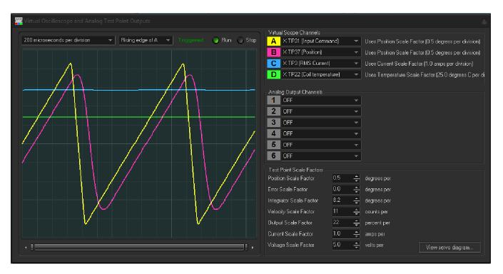
In this case, the coil current is 2.9 amps RMS and coil temperature is around 32 degrees C. The scanner will be dissipating 10 watts, and power required from the power supply is around 1.6 amps per rail.
