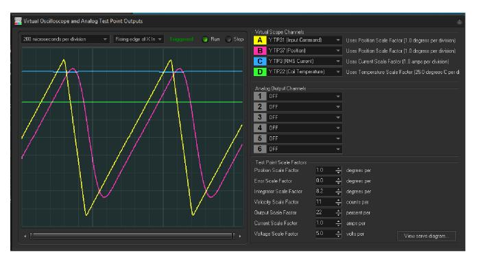
In this case, the coil current is 3.8 amps RMS and coil temperature is around 50 degrees C. The scanner will be dissipating 26 watts, and power required from the power supply is around 2.2 amps per rail.
