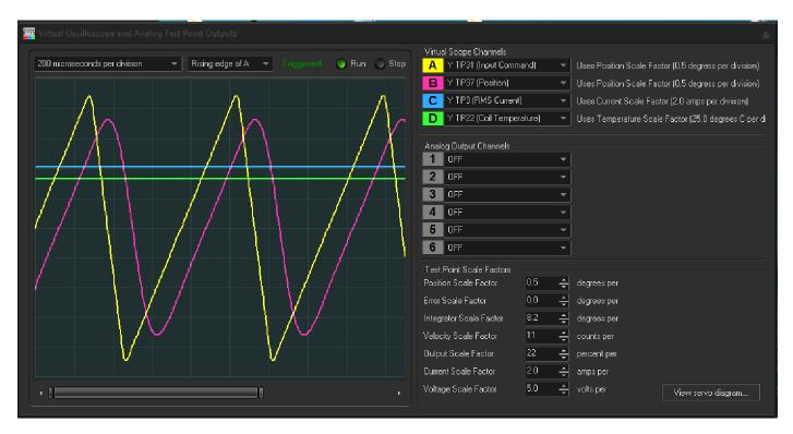
In this case we see that the RMS current being driven into the scanner is just above 4 amps, and coil temperature is still around 35C (assuming the scanner body is 30C). The scanner will be dissipating 16 watts, and power required from the power supply is around 2.25 amps per rail.
