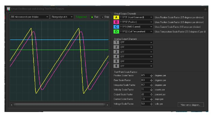
In this case, the coil current is 2.7 amps RMS and coil temperature is around 32 degrees C. The scanner will be dissipating 7.3 watts, and power required from the power supply is around 1.5 amps per rail.
