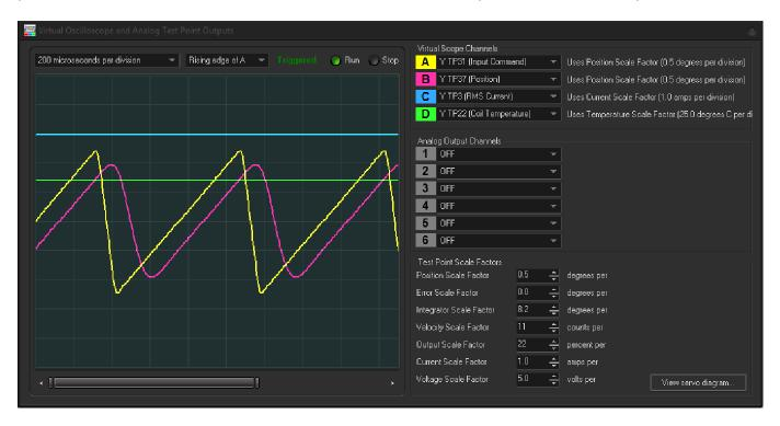
The oscilloscope shows that the RMS current being driven into the scanner is almost 3 amps and coil temperature is only around 35 degrees. Note that at this current, the scanner will be dissipating 9 watts of heat, which is certainly manageable. Power required from the power supply is around 1.8 amps from each of the +24V and -24V supply rails.
