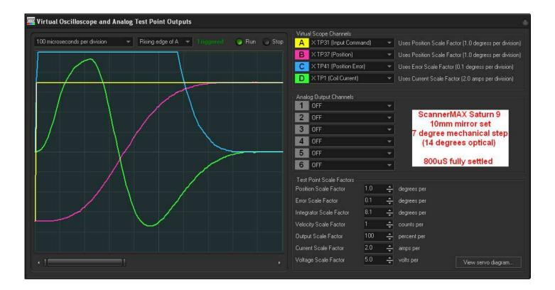
This is our standard Saturn 9 scanner with our mirror set capable of projecting 10mm beams over 40 degrees optical in both vertical and horizontal. This particular mirror set is made for vector scanning, so both X and Y mirrors have the same inertia (something unique to ScannerMAX scanners).
